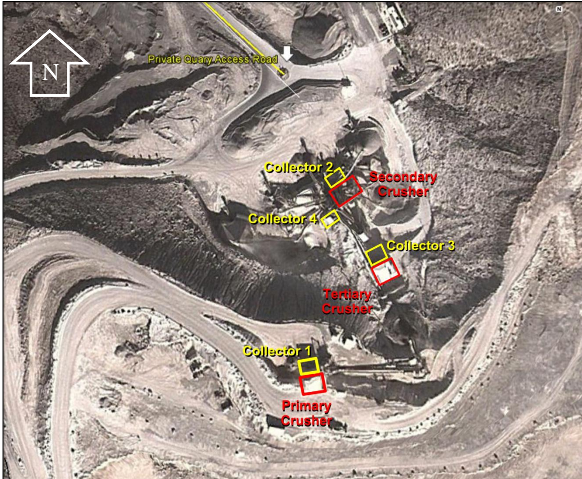
Figure 2.5 Google Earth Image of Cerro Mexico Quarry Indicating the Location of Crushers, Conveyor System and Dust Collectors
