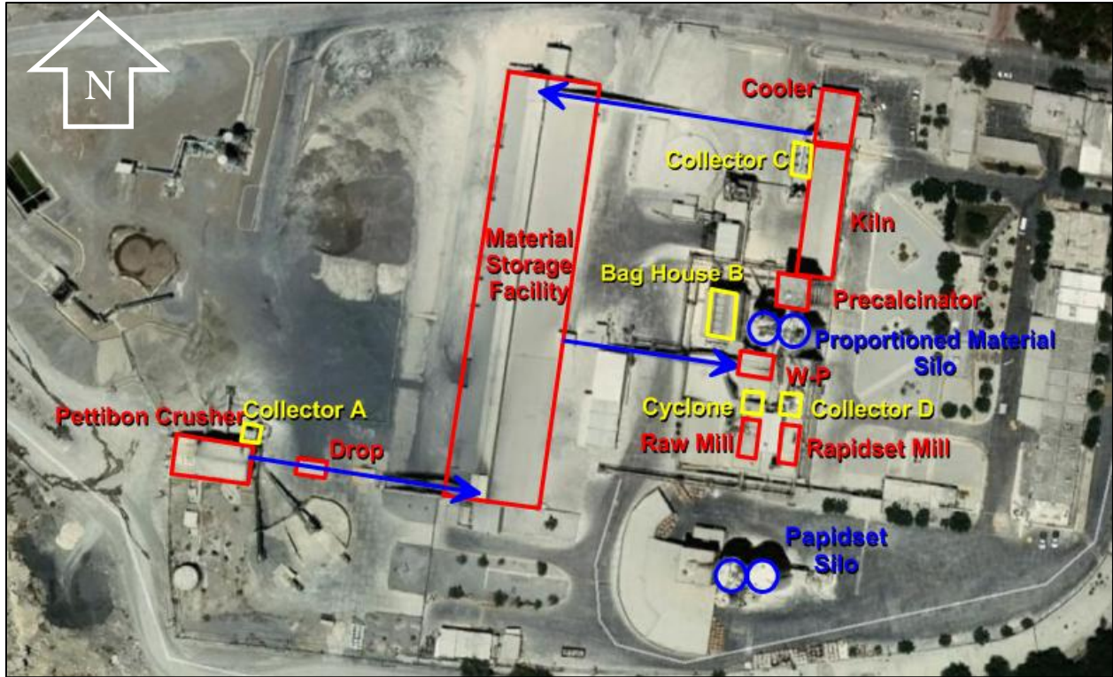
Figure 2.8 Google Earth Image of Juarez Cement Plant Indicating Main Facilities and Equipment
