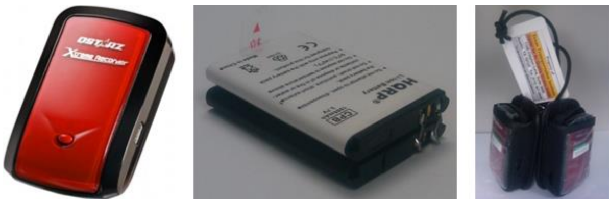
Figure 6: QStarz BT-Q1000eX Unit (Left); Extended Battery Pack (Middle); and Data Loggers Prepared for Testing (Right).
